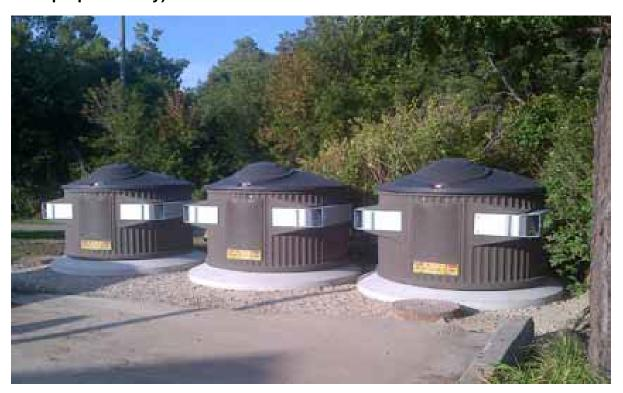
Second, the container holds more waste in a smaller footprint than a standard steel dumpster because much of the storage capacity is hidden underground. For example, 42% of the EnviroWirx's storage capacity is underground, which helps to disguise the actual mass of the container.
